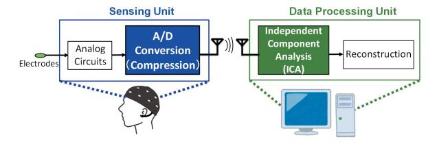
Compressed sensing allows compressing while sampling the signal, reduces the amount of information handled by the circuit, and thus enables low power consumption of the circuit. This leads to smaller battery size and longer operation time. However, general compressed sensing has the problem of being vulnerable to disturbances, which reduces the accuracy of reconstruction.
